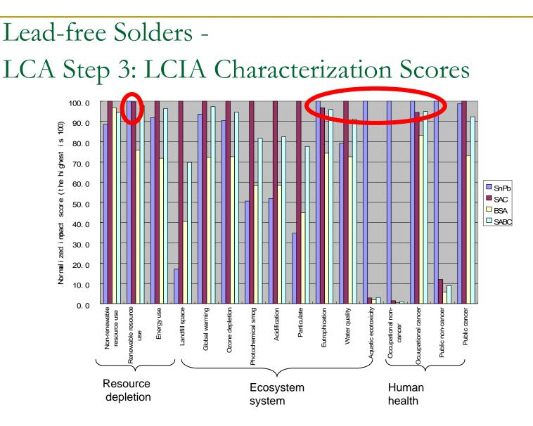
Normalized Life Cycle Assessment (LCA) impact score for paste Pb-free solders (Higher value indicates higher environmental impact); SAC: SnAgCu; BSA: BiSnAg, SABC: SnAgBiCu
